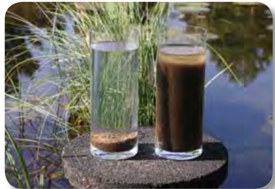
SVI s comparison of aerobic granular sludge (left) and conventional activated sludge (right)
